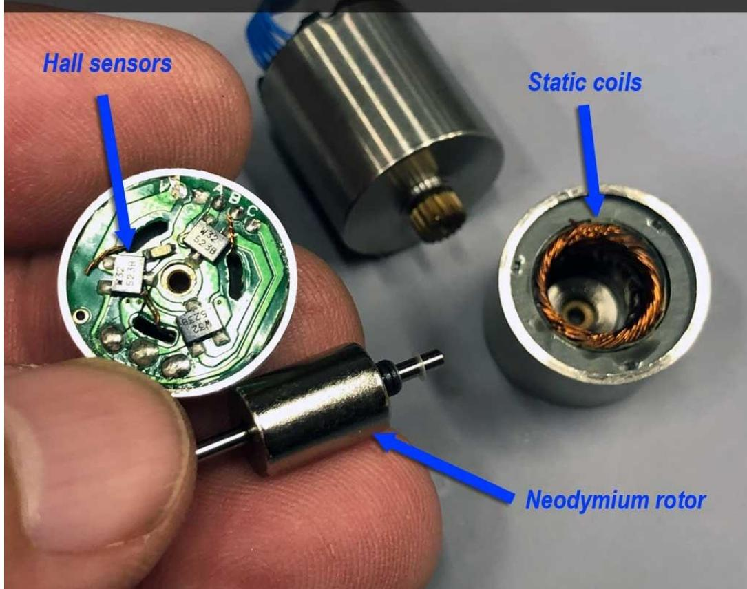
Principal advantage of brushless motors vs. coreless motors is the mere fact there are no brushes to wear out! This means the motor lasts longer. Much longer. So much longer!
