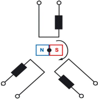
Brushless motors are also known as electronic motors. The all sensors measure magnetic fields so that the position of the rotor can be computed and the driving voltages to the coils (windings) can be adjusted. Thus, the Hall sensor literally measures the position of the rotor based on magnetic fields . . . meaning all it has to know is which sensor produces the highest reading!
