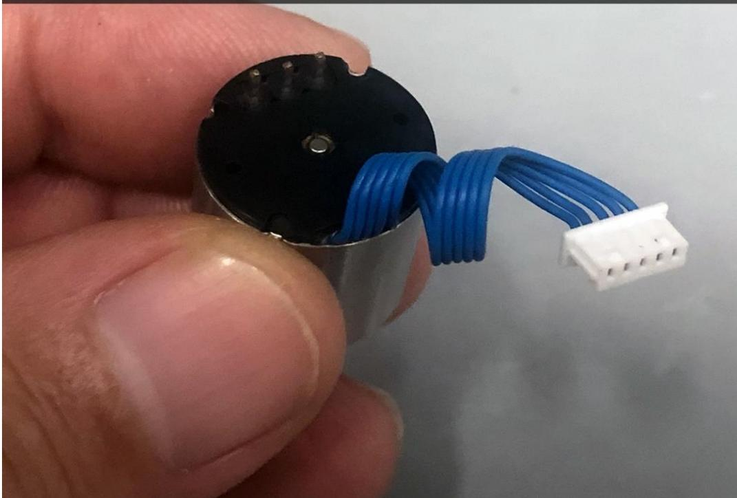
Next, note brushless motors are also wound using a mandrel. The point being, just like coreless motors, brushless motors are also used for high performance servos because they'll accelerate/decelerate more quickly than iron-core motors
