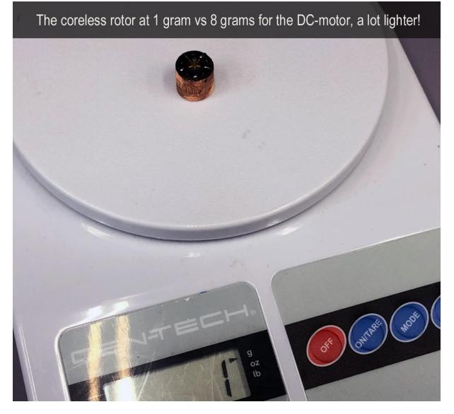
Bottom line? If speed matters, coreless beats DC every time because the mass being started and stopped is 'greatly' reduced. Commutation is still mechanical by a commutator ring and brushes. This means they wear out eventually but the brushes are a lot smaller.
