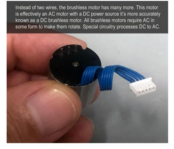
Next, note brushless motors are also wound using a mandrel. The point being, just like coreless motors, brushless motors are also used for high performance servos because they'll accelerate/decelerate more quickly than iron-core motors
