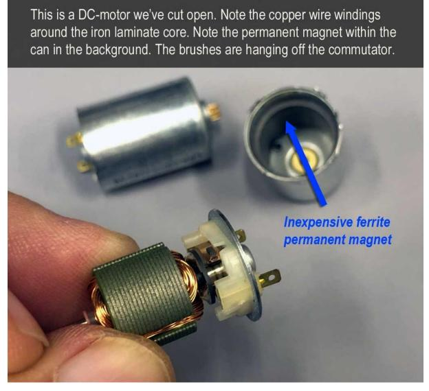
Sequentially turning the windings on, thus making an electromagnet to react against the permanent magnet mounted within the can, is what moves the rotor around and around. Commutation (switching the fields on and off in a sequence) is what times the force that keeps the rotor turning.
