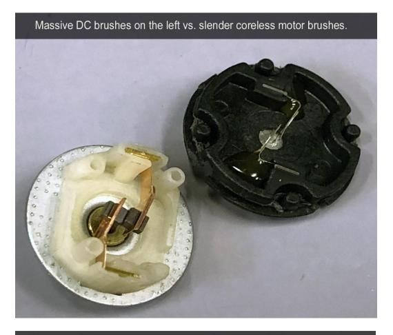
Note how the commutator ring is split. This is how sequential turning on-and-off of the windings work through the action of the brushes.
