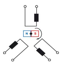
Brushless motors are also known as electronic motors. The all sensors measure magnetic fields so that the position of the rotor can be computed and the driving voltages to the coils (windings) can be adjusted. Thus, the Hall sensor literally measures the position of the rotor based on magnetic fields . . . meaning all it has to know is which sensor produces the highest reading!
