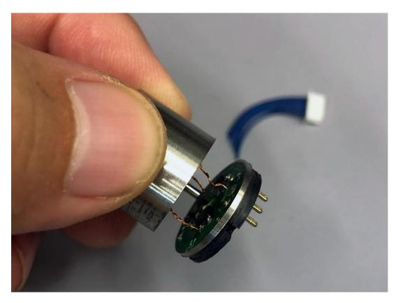
So what replaces the brushes? The answer to that is simple; what replaces brushes are Hall effect sensors. Their output voltage is directly proportional to the magnetic field strength through it. These are usually combined with threshold detection so that it acts as a switch.
